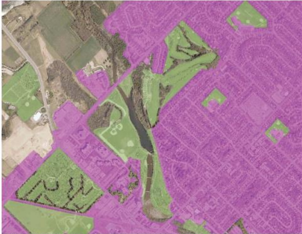
Fig 2: Impervious versus Pervious Areas for the WHPAs A, B and C areas
